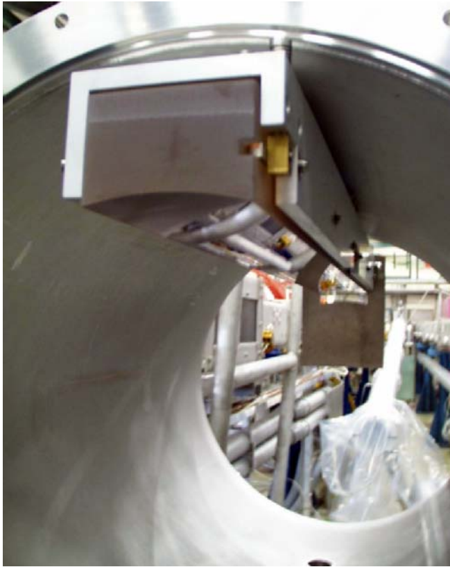
Fig. 6 View of the focusing mirror of the JCNS focusing SANS instrument
